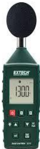
Figure 8: Noise measuring equipment used
